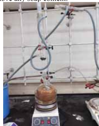
Figure 1. Transesterification process setup.
