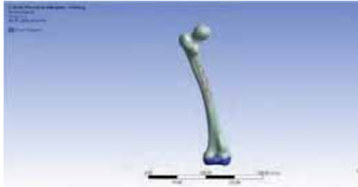
Figure 6. Applying Fixed Support
