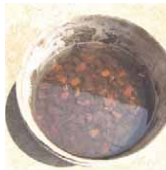
Figure 3. Soaking Burnt Brickbats in water.
