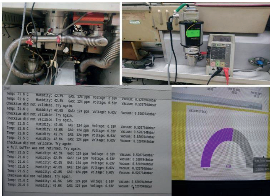
Figure 3. Vacuum Readings (mbar) on UI and Alert
