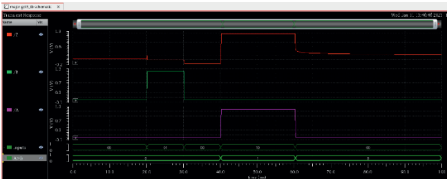
Figure 11. Simulation of GDI based comparator for A < B , A = B and A > B
