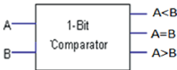
Figure 1. Block diagram of the comparator
