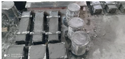
Figure 1. Casting of Cube, Cylinder & Prism Specimen
