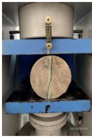
Figure 5. Failure of Cylinder
