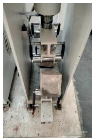
Figure 7. Failure of Prism
