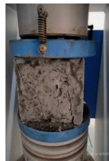
Figure 3. Failure of Cube
