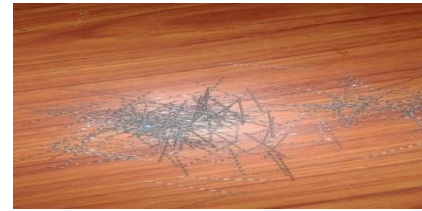
Figure 1. Crimped steel fibers
