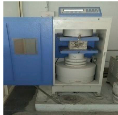
Figure 2. Compressive testing machine
