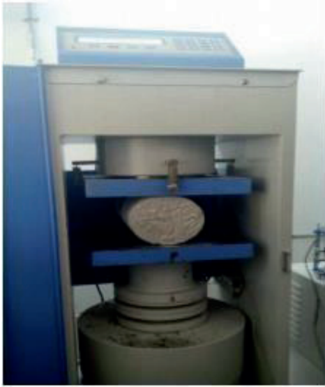
Figure 3. Split Tensile testing machine.
