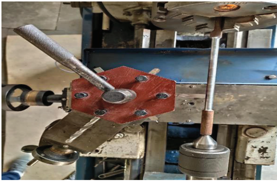
Figure 14. turret holding four single point cutting tools, one drill bit of 8mm, one forming tool
