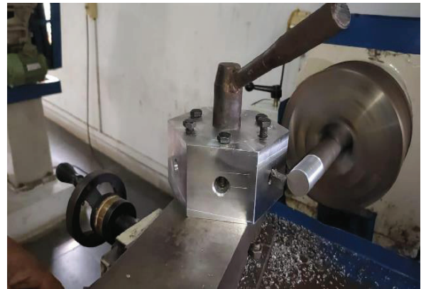
Figure 11. the above figure show the simple turning operation of a rod of 28mm diameter
