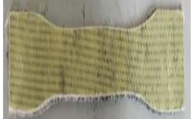
Figure 2. Test specimen for tensile testing in Universal testing machine
