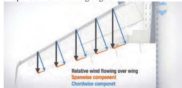
Figure 4. Swept wing spanwise flow
