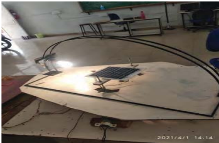
Figure 15. Solar panel and incandescent bulb setup
