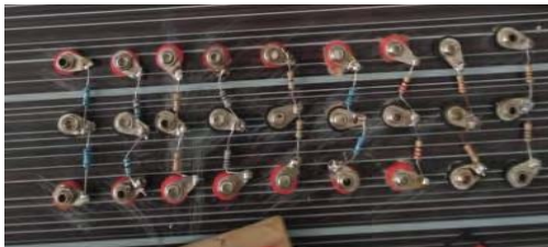
Figure 17. Resistive load as per requirement
