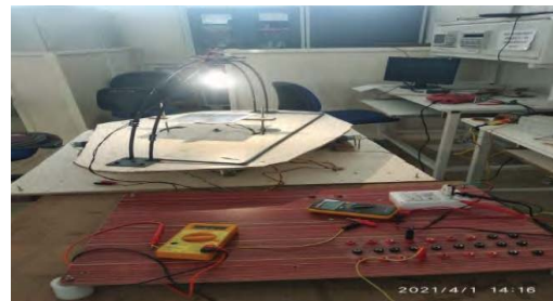
Figure 20. Snapshot of solar power measurement.
