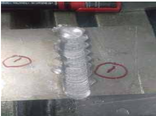
Figure 9. Slab welded at 30 mm
