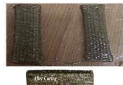
Figure 6. Additively manufactured specimen of Kevlar composite
