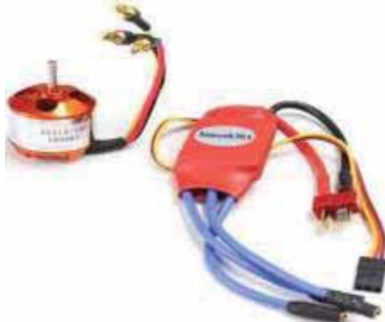
Figure 5. BLDC motor with Electronic Speed Controller
