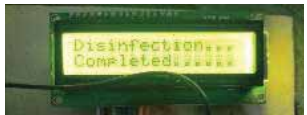
Figure 20. After disinfection time is passed, message as disinfection Completed is shown and Buzzer is ON and tray gets open.
