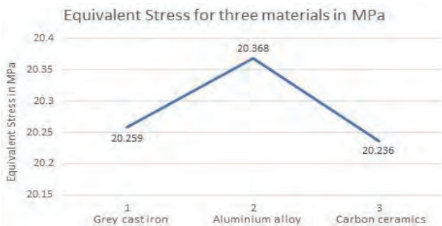
Figure 14. Equivalent Stress Graph for Different Materials
