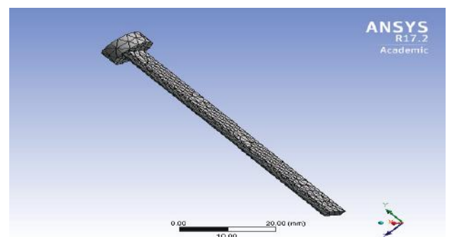
Figure 17. Meshing of the oblong punch (Tetrahedron 10-nodes)
