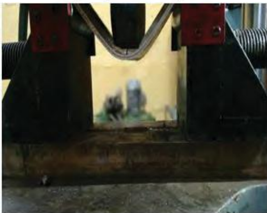
Fig-7 Bend test setup
