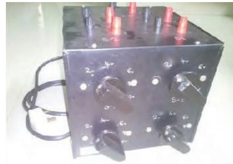
Figure 2. Transformer with five output voltages (2V, 4V, 6V, 8V, 10V)
