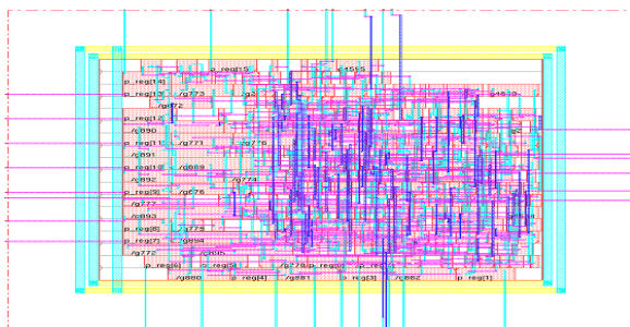
Figure 14: Final layout design of modified Booth multiplier.
