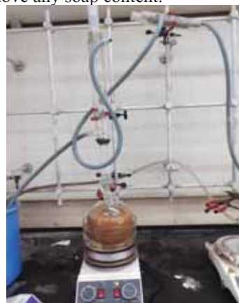
Figure 1. Transesterification process setup.
