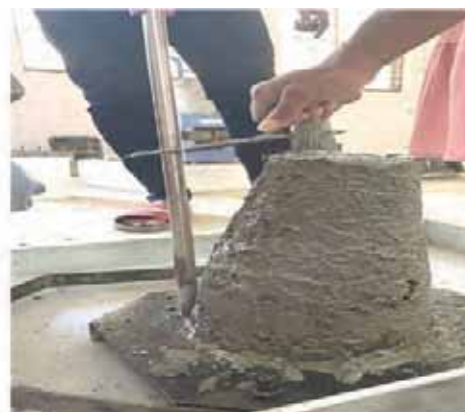
Figure 8. Workability by Slump Test
