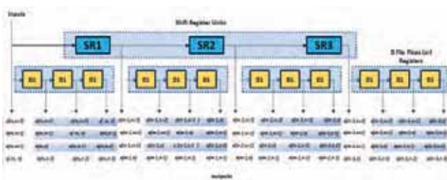
Fig.1. Data flow in the fully direct form structure for N=4 with four outputs \{y(m, n), y(m, n+1), y(m, n+2), y(m, n+3)\} , [10].
