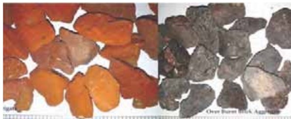
Figure 2. Difference between Normal Brick Bats and Over Burnt Brick Bats
