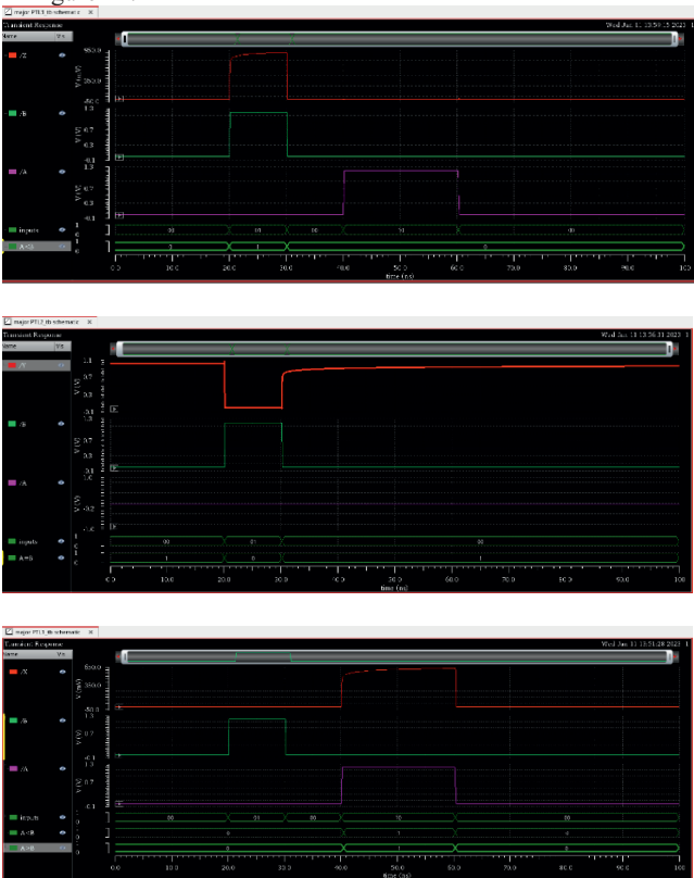
Figure 12. Simulation of PTL based comparator for A<B, A=B and A>B
