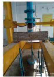
Figure 9. Failure of Beam
