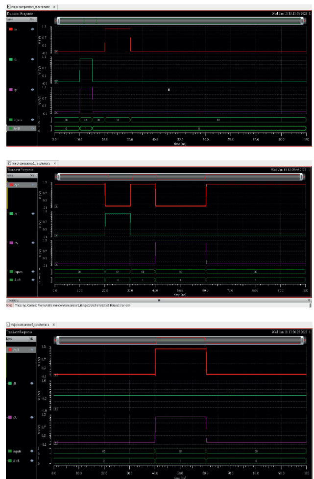
Figure 10. Simulation of CMOS comparator for A < B , A = B and A > B
