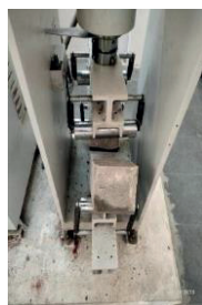
Figure 7. Failure of Prism
