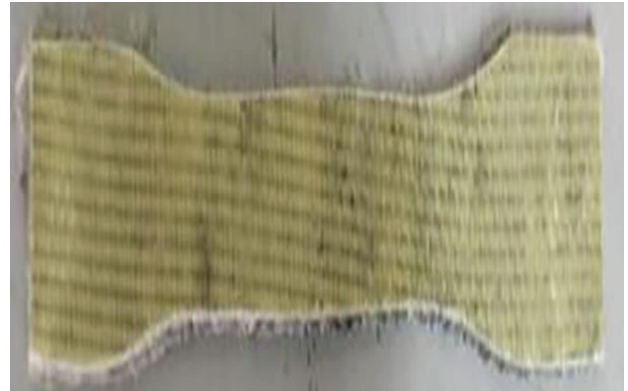
Figure 2. Test specimen for tensile testing in Universal testing machine
