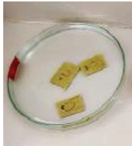
Figure 6. Test set up for water absorption
