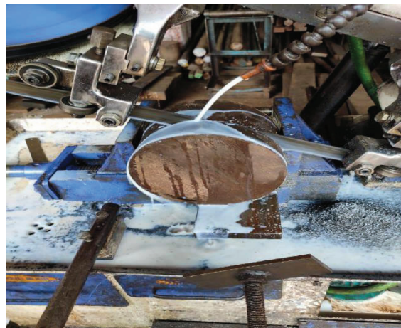
Figure 6. The above figure shows the cutting process of a mild steel block
