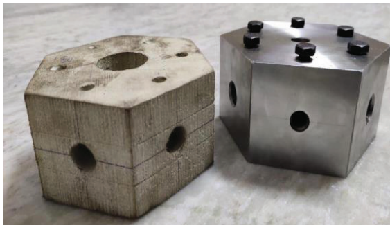
Figure 15. the above figure shows the comparison between foam and metal prototype
