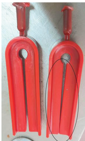
Figure 11. Camber, After Cooling to Room Temperature
