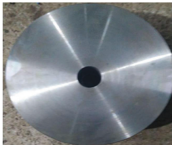
Figure 7. the above figure shows the block after the turning, facing and boring of MS block in lathe machine
