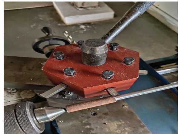
Figure 11. the above figure show the simple turning operation of a rod of 28mm diameter
