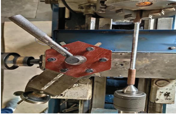
Figure 14. turret holding four single point cutting tools, one drill bit of 8mm, one forming tool
