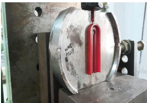
Figure 10. First Trial (Drag Half Removed)
