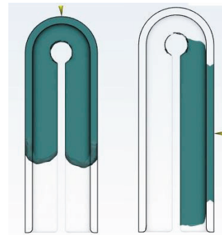
Figure 7. Fill Results in 3 Seconds, GP1 (L), GP2 (R)
