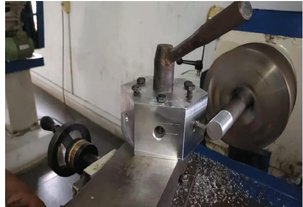
Figure 11. the above figure show the simple turning operation of a rod of 28mm diameter
