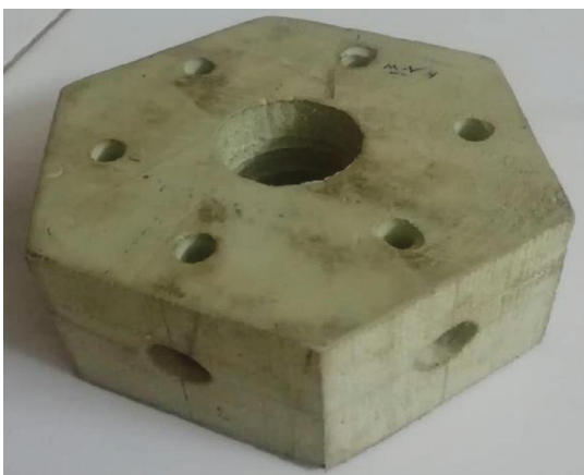
Figure 4 & 5. Prototype of turret made with foam
