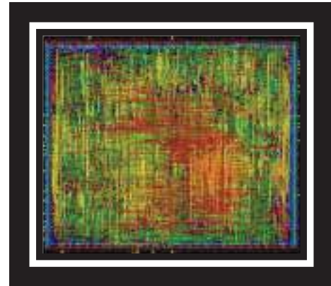
Figure 11. Physical design layout of proposed FIR filter architecture in 90 nm technology.
