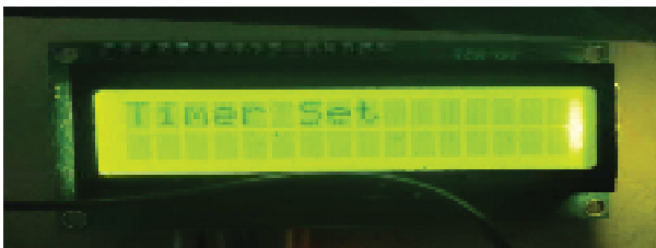
Figure 16. After time is set, displays it on the LCD as timer set.
