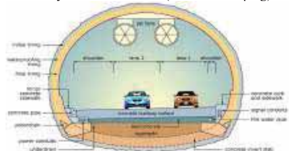
Figure 2. Cross-sectional view of a general tunnel
