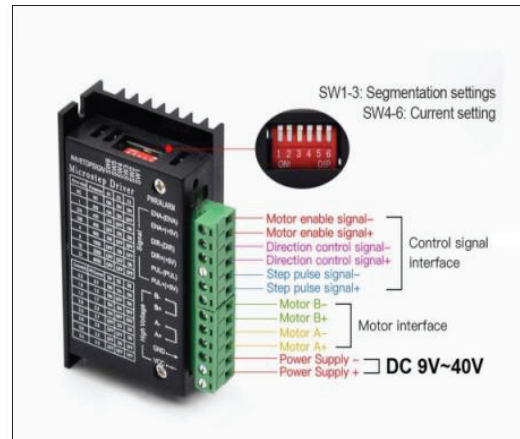
Figure 13. Stepper motor driver.
