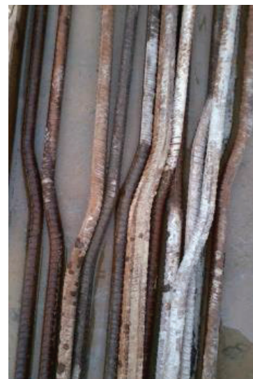
Figure 1. Profile of Rebar for lap splice
