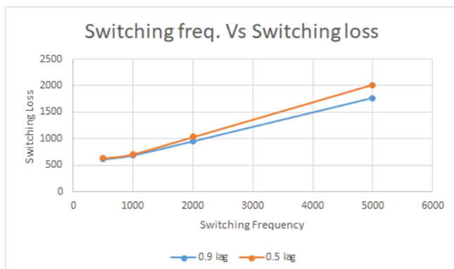
Figure 10. Switching frequency versus switching loss for CHBI
