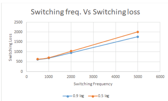
Figure 17. Switching frequency versus switching loss for DCMLI
