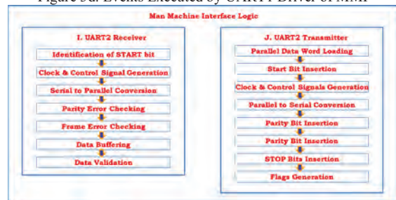
Figure 3e. Events Executed by UART2 Receiver & UART2 Transmitter Logics of MMI
