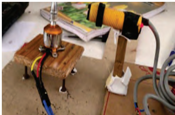
Figure 6. Finding the speed of the BLDC motor using the proximity sensor
