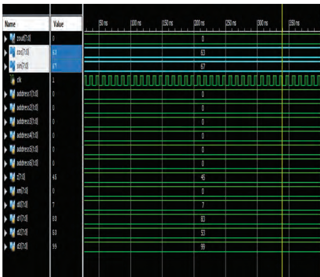
Figure 16. Simulation Result of Unrolled CORDIC using MUXes
