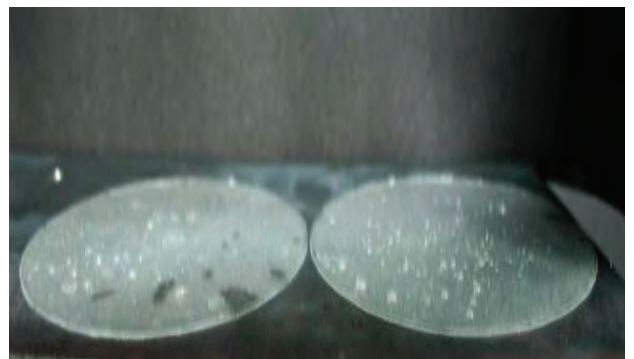
Figure 4. Dew formation on PDMS substrates.
