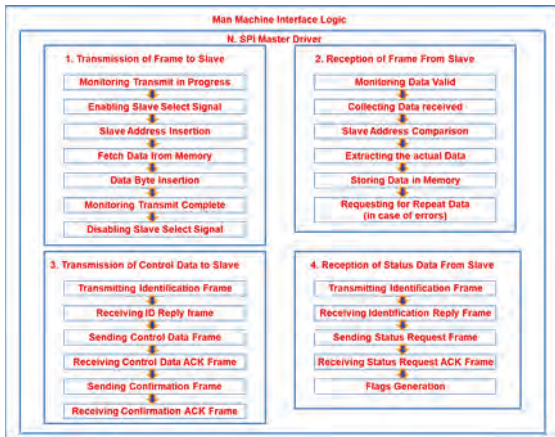
Figure 3h. Events Executed by SPI Driver Logic of MMI
