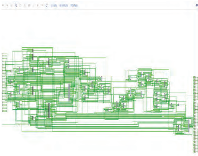
Figure 15. Schematic of Unrolled CORDIC using MUXes
