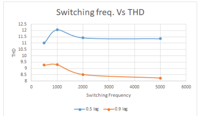
Figure 11. Switching frequency versus TDH of CHBI
