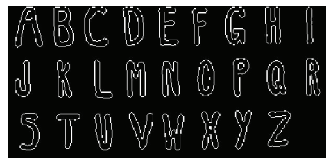
Figure 14. Edge detection of Fig. 2 gray image using zero-crossing of Laplacian of Gaussian filter
