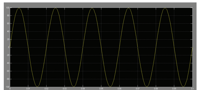
Figure 3. Simulink output display of the harmonic components waveform of the stage-1 inverter, after the output is filtered.
