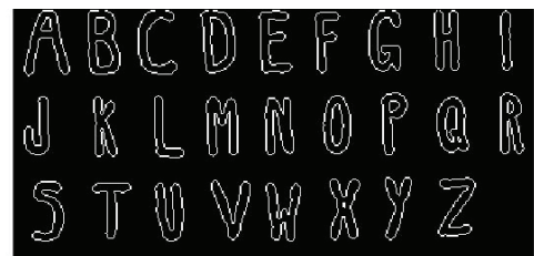
Figure 13. Edge detection of Fig. 2 gray image using the zero-cross method
