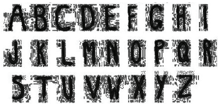
Figure 8. Contrast adjusted image of Fig. 2 gray image using histogram equalization
