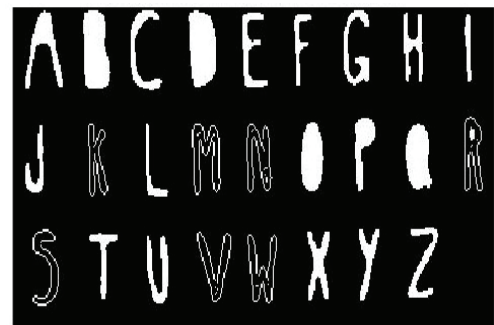
Figure 18. Thin image of the edge detected image Fig. 15 after image filling
