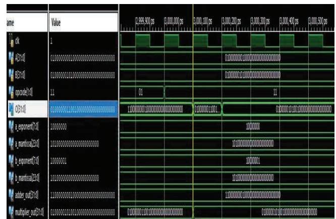
Figure 12. Simulation Waveform for FPU in FPGA
