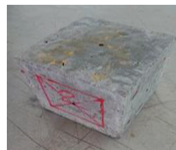
Figure 6(a). Cube after 02 hrs. in High Temperature Furnace at 200°C
