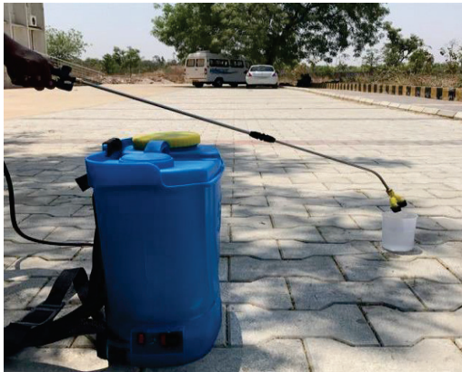
Figure 4. Measuring the flow rate of standard flat fan nozzle using a measuring flask
