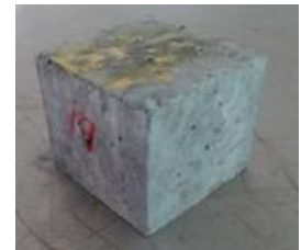
Figure 5. Cube after 02 hrs. in High Temperature Furnace at 100°C
