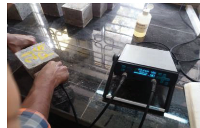
Figure 2. Ultrasonic Pulse velocity measurement of cubes
