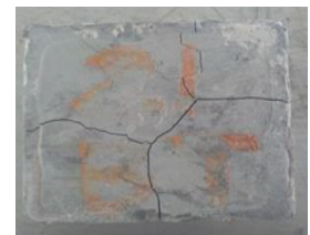
Figure 7(b). Cube after 02 hrs. in High Temperature Furnace at 500°C
