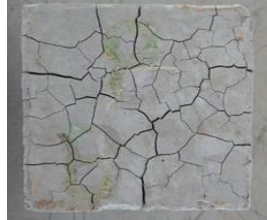
Figure 9(b). Cube after 02 hrs. in High Temperature Furnace at 900°C
