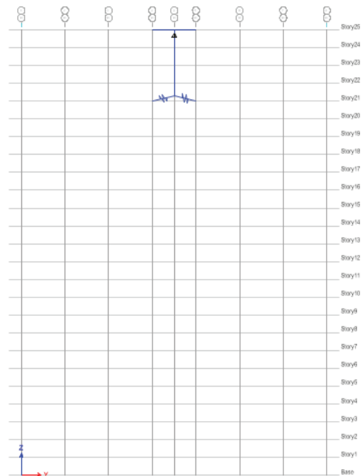
Figure 1. Elevation of the building with Tuned Mass Damper placed at centre
