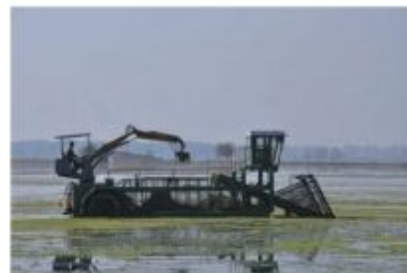
Figure.10. A Dewatering machine removing aquatic weeds
