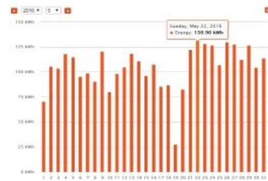
Figure 13. Energy generated by Single axis tracking-20kW String Inverter output on 22 nd May '16
