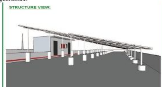
Figure 8. 3-D view of Single axis polar tracking plant
