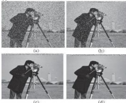
Figure 4: Images received at the OFDM receiver with BPSK technique for (a) SNR=0 (b) SNR=5 (c)SNR=10 (d)SNR=20
