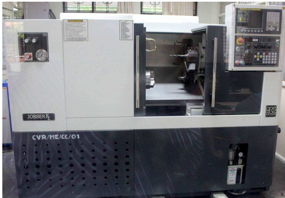
CNC Horizontal Turning Center (Make: Ace Designers)
