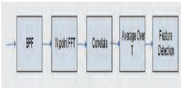
Figure 6. Cyclostationarity Feature Detector
